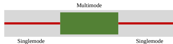
Fig. 1 SMS structure fiber optic sensor configuration.
